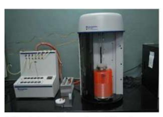
Surface Area is an intrinsic property of powdered porous materials that can reveal important information regarding the usefulness of a material for an application, Surface area plays critical role in the bio-availability of Pharmaceuticals, dispersion of dyes, adsorption capacity of carbon and many more. Surface area analyser is used for surface area measurement by means of Physical adsorption.
