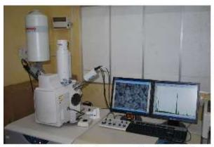
Scanning electron microscopy (SEM) uses a focused electron probe to extract structural and chemical information point-by-point from a region of interest in the sample. The high spatial resolution of an SEM makes it a powerful tool to characterize a wide range of specimens at the nanometer to micrometer length scales.
