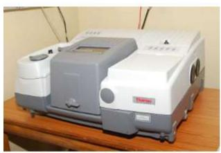
Infrared spectroscopy technique based on the vibrations of the atoms of a molecule. An infrared spectrum is commonly obtained by passing infrared radiation through a sample and determining what fraction of the incident radiation is absorbed at a particular energy. The energy at which any peak in an absorption spectrum appears corresponds to the frequency of a vibration of a part of a sample molecule.
