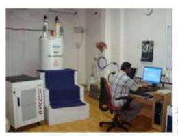
Nuclear Magnetic Resonance (NMR) is a powerful non-selective analytical tool that enables you to ascertain molecular structure including relative configuration, relative and absolute concentrations, and even intermolecular interactions without the destruction of the analyte.
