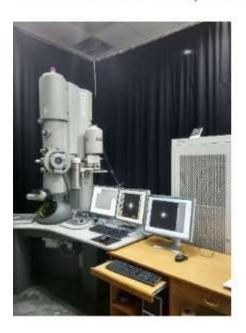
An Electron Microscope uses an electron beam as a source of illumination and the electromagnetic lenses to manipulate the beam to penetrate the sample. The resulting diffraction pattern reveals the structure of the observed sample.
