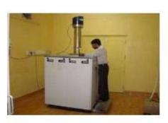
Gamma chamber 5000 is a compact, portable, self-shielded type of a Co-60 Gamma Irradiator. Its design conforms to American National Standards ANSI-N433.1, 1977 for safe design and use of self-contained Dry Source Storage Gamma Irradiator (category-1) Atomic Energy Regulatory (AERB), India.
