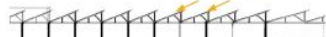
Fig: North light windows in the weaving sheds allow the North light to come inside the structure
