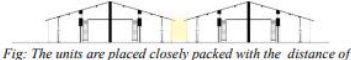
Fig: The units are placed closely packed with the distance of 1.5 m keeping the streets shaded
