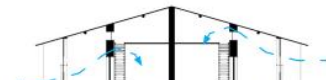
Fig: The section of chaali unit showing the air circulation inside the unit
