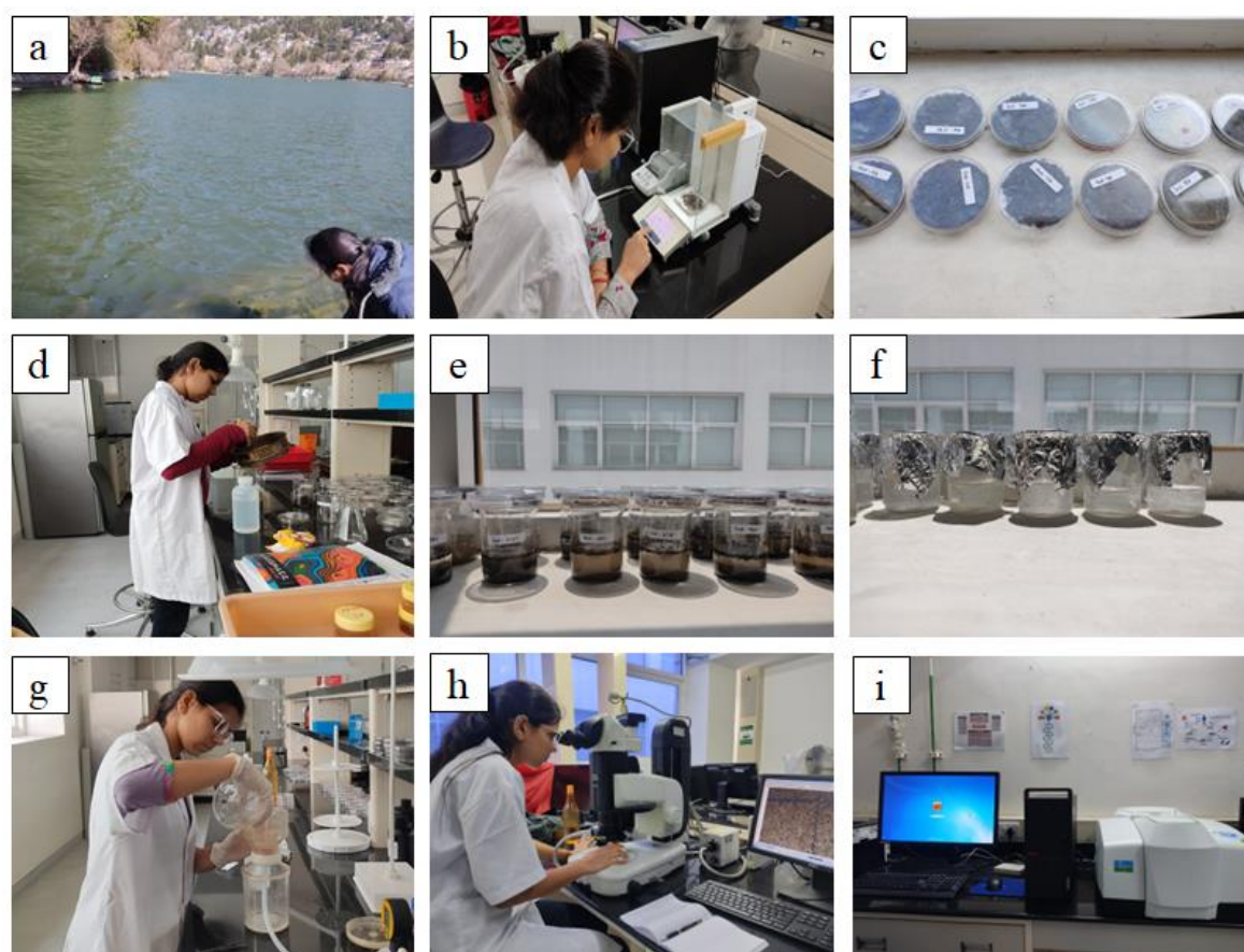
Fig. 3.6 Pictures representing the steps followed during the procedure: (a) Sample collection; (b) Sample weighing; (c) Sample drying; (d) Sieving; (e) Density-separation; (f) Organic digestion; (g) Filtration; (h) Microplastics analysis (quantitative); and (i) Qualitative analysis using FTIR
